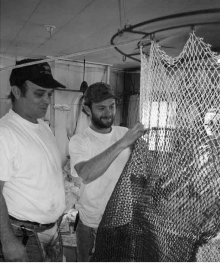
Fig. 5.2. James Golden and his nephew Michael Holton stitch a mandated Turtle Excluder Device (TED) into a net. Turtles hit the metal platform and slide out through a hole in the net. Photo by Faith Eidse.
