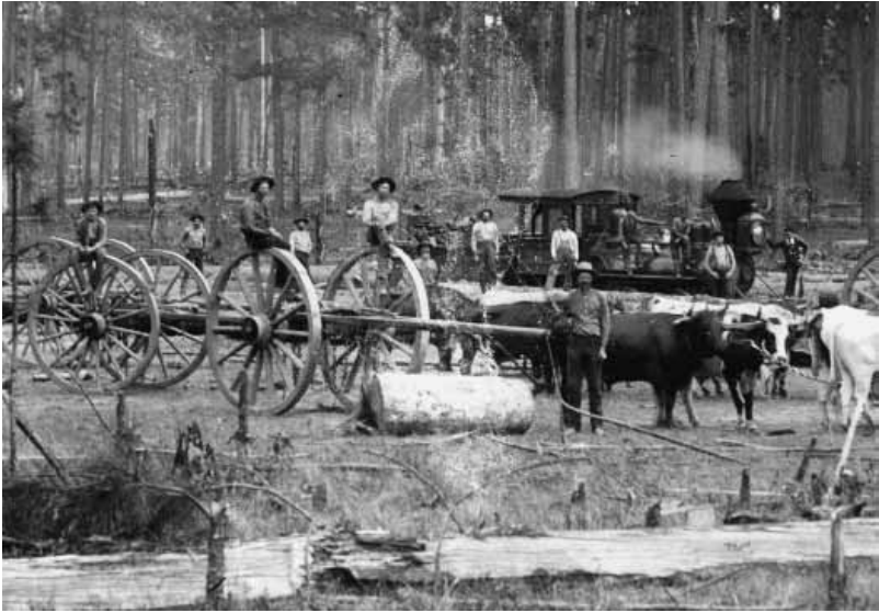
Fig. 7.1. A logging crew uses caissons (high-wheeled ox carts) and a locomotive to clear woods in 1900s Florida. Photo courtesy of Florida State Archives.
